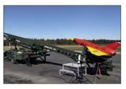
Robonic Ltd Oy is the world's premier UAV/RPA launch systems house. Robonic has more than three decades of operational experience with pneumatic technology to achieve zero point or short rail
